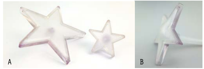
Figure 10. Star buttons fabricated with auxiliary support (A). The big star is inflated in (B) at 0.6 psi (4.1 kPa) relative to atmospheric pressure.
