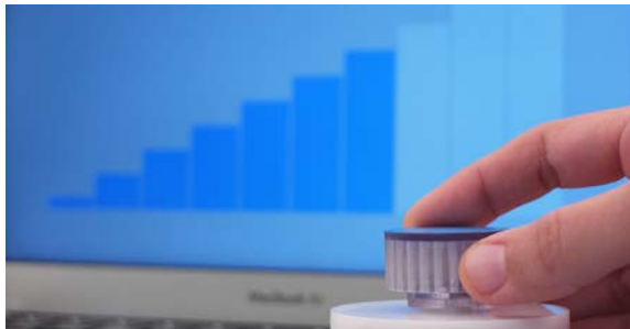
Figure 19. We use the sawtooth knob of Figure 14 to control volume in a prototype application. The current volume level is rendered real-time on the screen (as in the background of the image).
